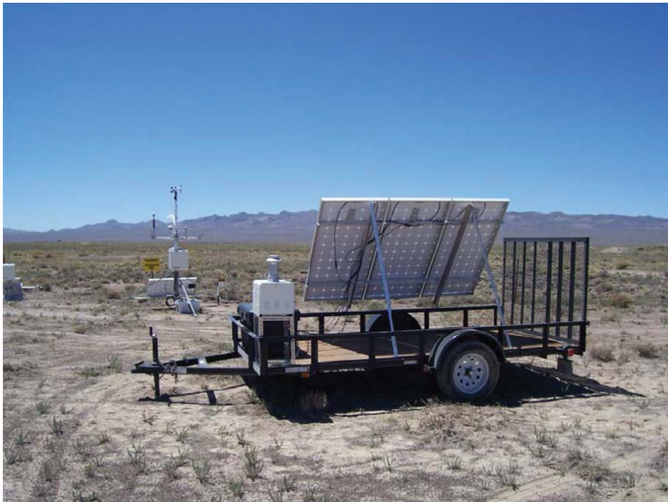
FIGURE 1-6. Station 402 consists of a trailer mounted solar powered air sampler and a portable meteorological tower located on the north fenceline at Clean Slate 1.
