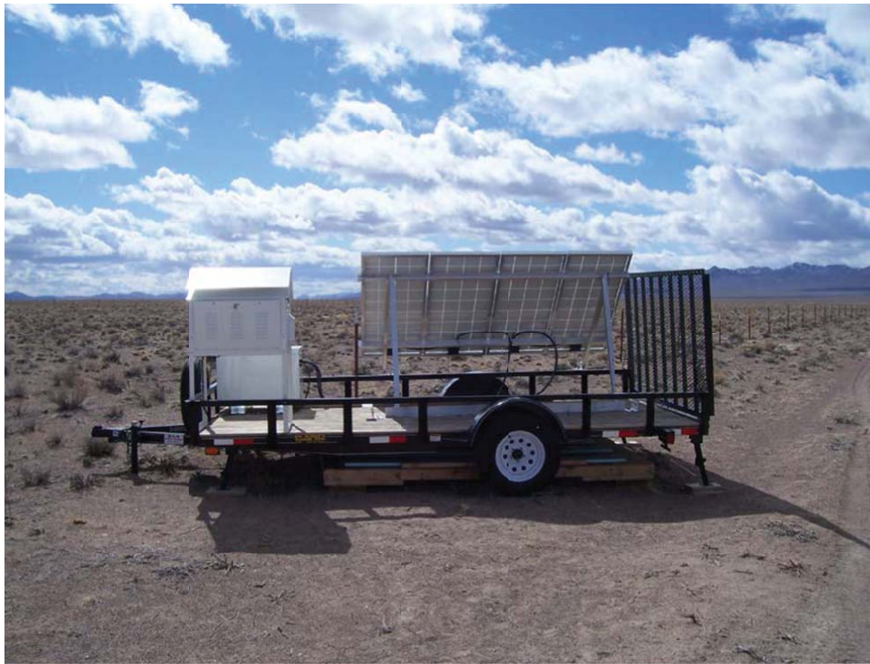
FIGURE 1-4. Station 401 includes two solar powered air particulate samplers mounted on a trailer for mobility and is positioned on the north fence of Clean Slate 3.
